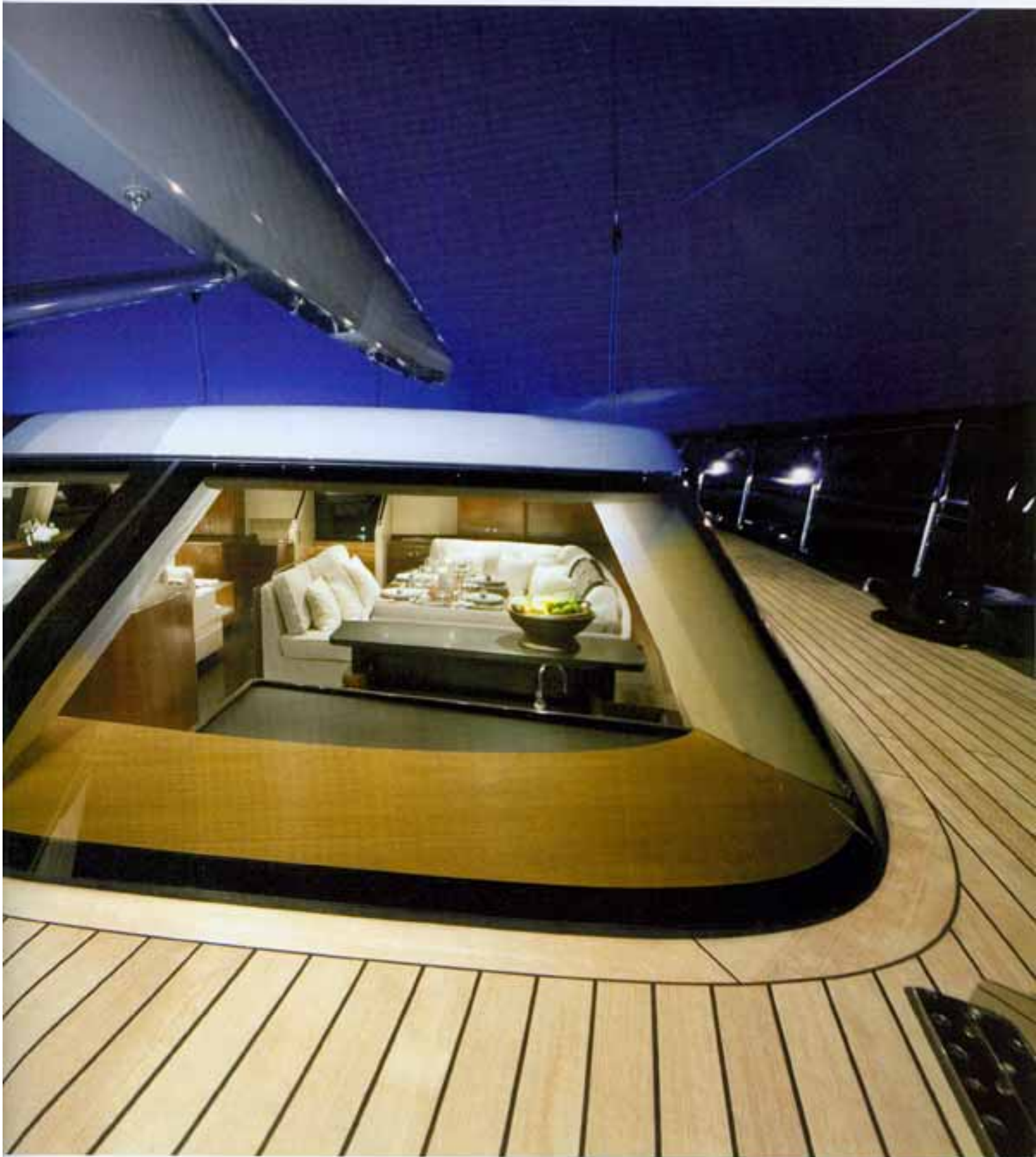
Unusually, Mystère's saloon windscreen meets the deck directly without the usual visible frame of a raised coachroof, enhancing her clean lines by creating the illusion of a single deck level flowing around the length of the yacht
